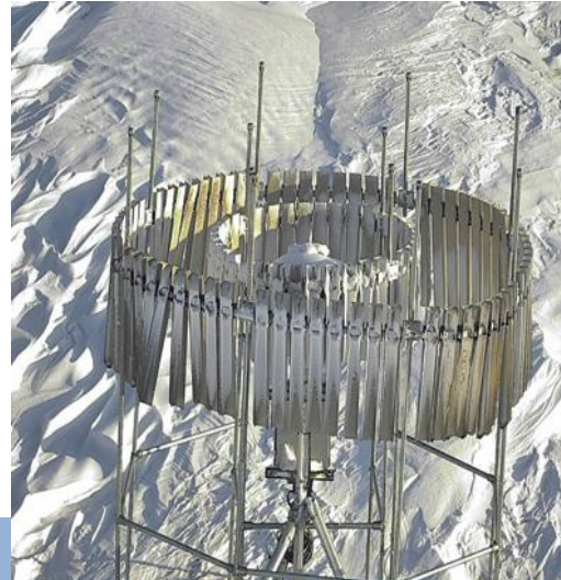
Multi-Angle Snowflake Camera (MASC)
