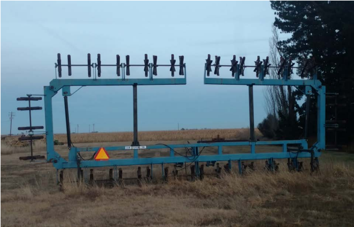
Figure 2. Picture of sand fighter implement used to prevent wind erosion from damaging young cotton plants or soil blowing away.
