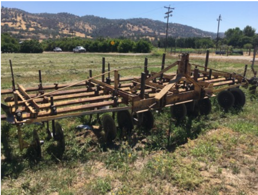
Image 5: A tractor implement made by Full Belly as part of their minimum till efforts. The implement allows them to move cover crop residue out of the way in order to plant without further disturbing the soil.
